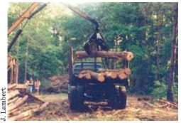
A knuckle boom-loader places pine logs on a truck in a first-time thinning operation for a 16-year-old plantation. As Lambert removes loblolly pines, he plants longleaf.
